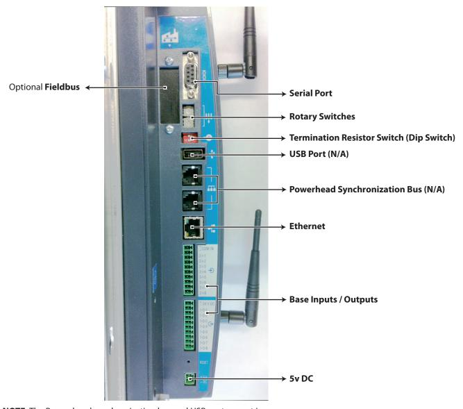
**NOTE:** The Power-head synchronization bus and USB port are not in use.
